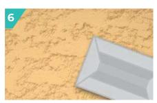
"Crushed rough" finish: Crush the grain using a float before it hardens.
