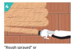
"rough crushed" finish: Spray a 1st application of render to a thickness of 10 mm. Smooth the 30 x 20 cm glass
